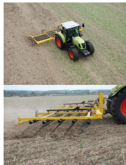
The Straw Harrow consists of five banks of hard-wearing double-coil spring tines, the angle of which can be hydraulically altered in order to achieve a more 'aggressive' action, and can typically be used at a high operating speed of up to 25 kph, so allowing outputs of around 12ha/hour to be achieved.
