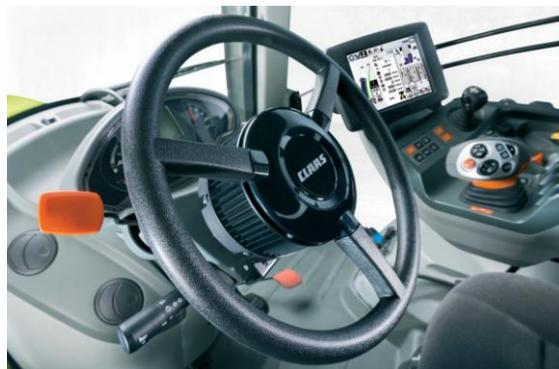
Installation could not be simpler as the control system is fully integrated into a control box and steering wheel that is fitted in place of the normal steering wheel. Having removed the steering wheel and replaced it with the GPS PILOT FLEX steering wheel, steering commands are sent directly to the steering wheel's electric motor and so directly to the steering linkage.
