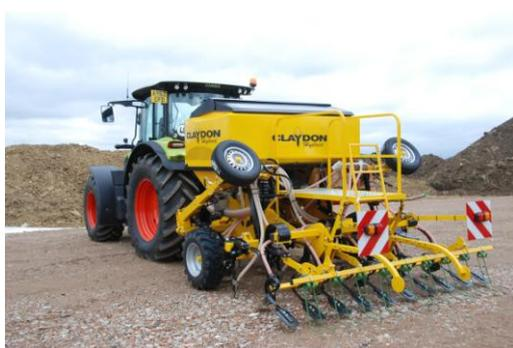
*The new Claydon 3.0m drill with split hopper*
