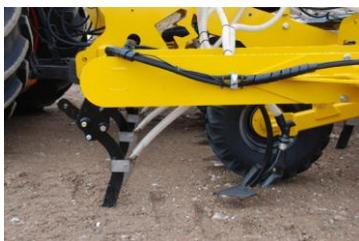
In standard format, the fertiliser is fed down the back of the leading rigid chisel breaker tine and is placed 75-100mm below the seeding zone so that it is perfectly placed for the young seedling. However, if required the design also allows for the fertiliser to be fed down the back of the seeding tine, so that it is mixed with the seed, or placed on the surface.
