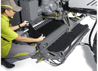
Both QUADRANT balers also feature the hydraulically-lowered drop-floor in the cutting chamber, which is lowered automatically if the unit is overloaded. This enables the driver to remove any possible blockages at the baler intake simply by reducing the PTO speed from the driver's seat, and continue baling without interruption or problems. The driver does not have to get out to perform laborious manual clearance.
