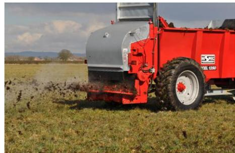
As part of its standard specification, the new XCEL 1250 is fitted with a wide angle PTO, driving a 200hp rated gearbox, and the spreader's main transmission system is protected by an over-run clutch and shear bolts.
