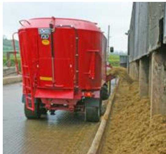
The VHD conveyor comprises of a modular conveyor belt and elevator, which can be extended out either side of the feeder by up to 26cm, making it ideal for central feed passages where turning round is difficult.
